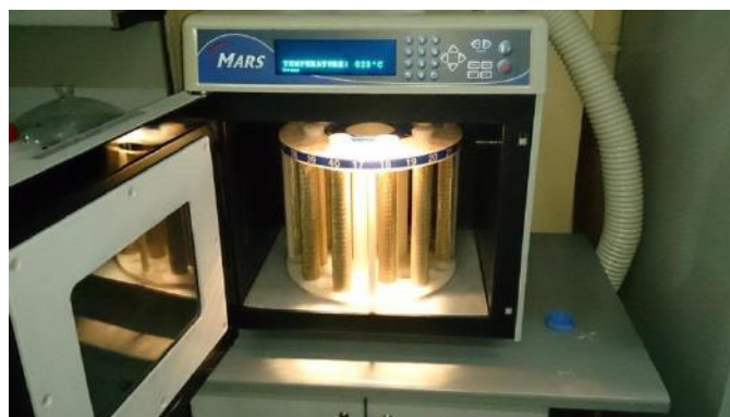
Figure 1. Reduction of graphene oxide by hydrazine hydrate under microwave irradiation (MWI)
