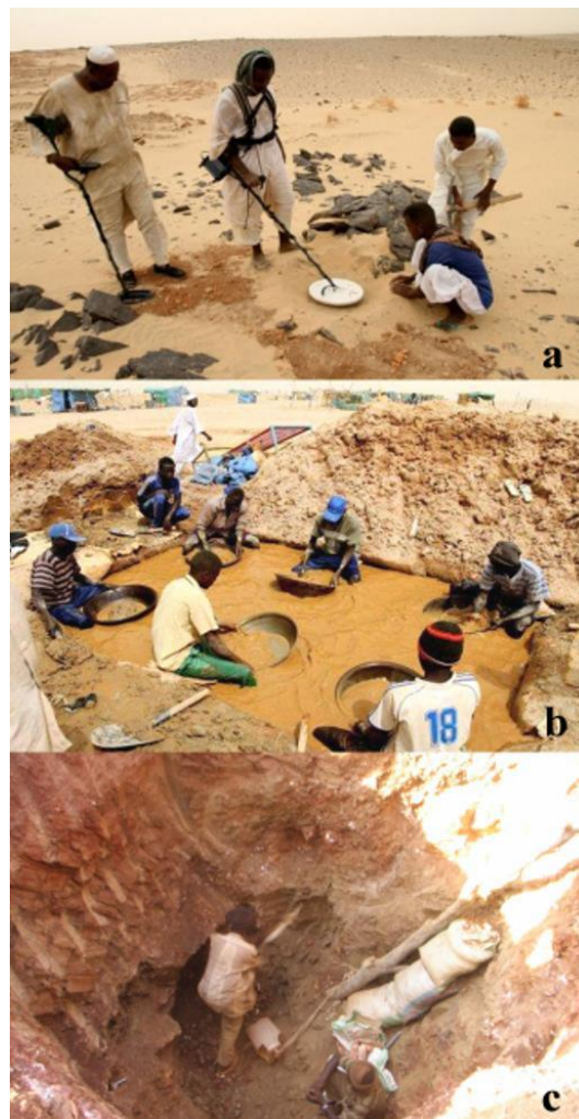
Figure 4. (a) mining with metal detector devices, (b) mining using sieves, (c) open pit mining.
