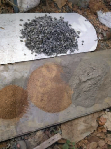
Figure 7.1: Ingredients of concrete mix
