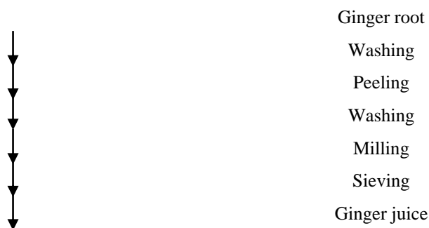
Fig 2.0 Flow diagram for the production of ginger juice from ginger root. Sasi et al. (2013)
