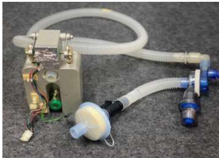
Figure 2. The two double-acting pistons pump system in experimental tests.
